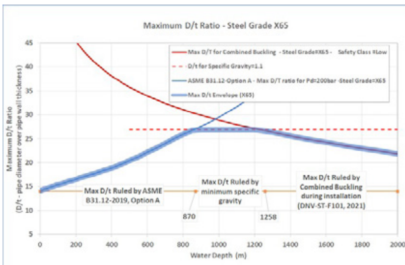
Picture 6 – Example of Sizing Criteria applicable to hydrogen offshore pipeline design as a function of water depth
