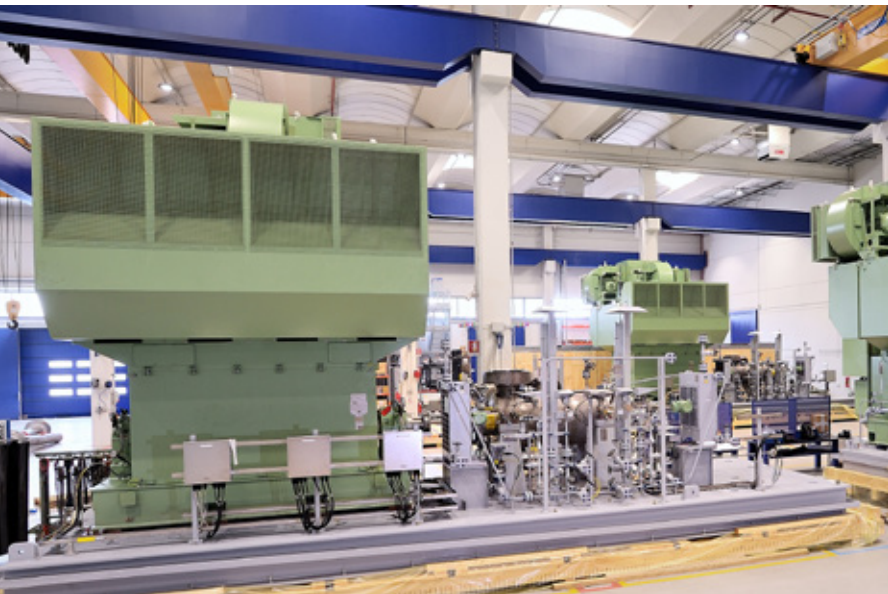
API 610 BB5 Water Injection pump unit - final skid assembly at Trillium's Italian facilities (Nova Milanese)
