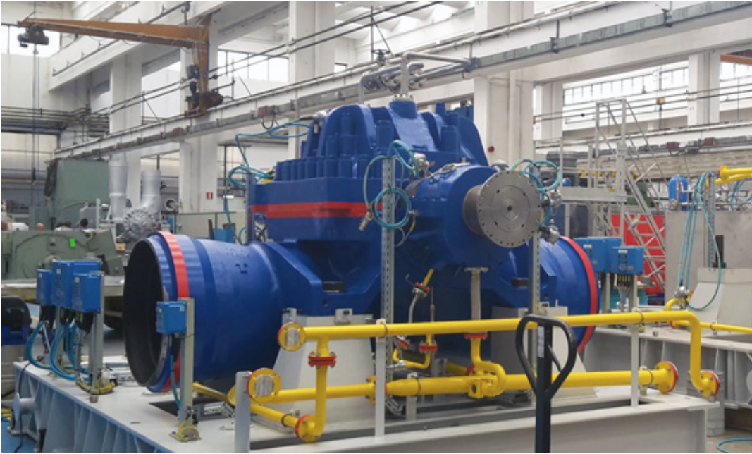
API 610 BB1 MOL pump - final skid assembly at Trillium's Italian facilities (La Spezia)
