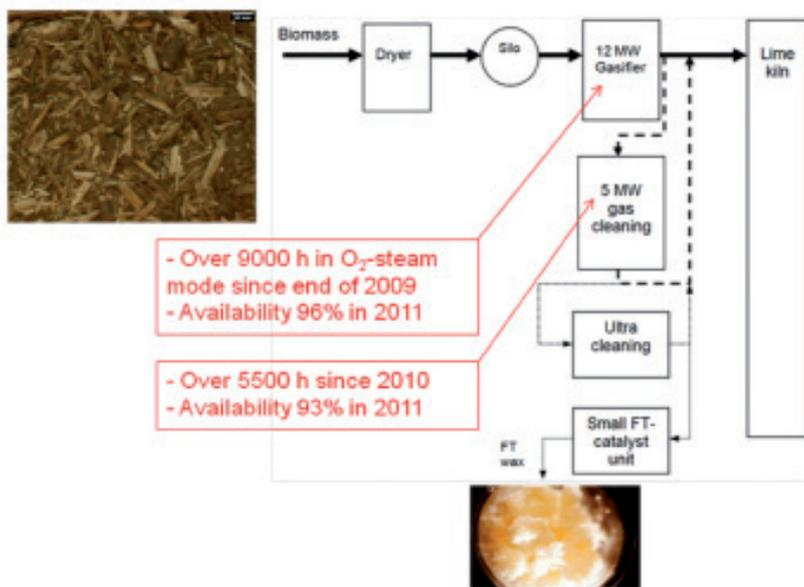
Fig. 5 - Process chain of the NSE demo plant
