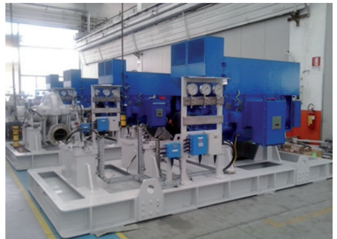
Fig. 4 – Induction motor CT 400 Y4 type at the Termomeccanica Pompe facilities, mounted onto the BP skid
