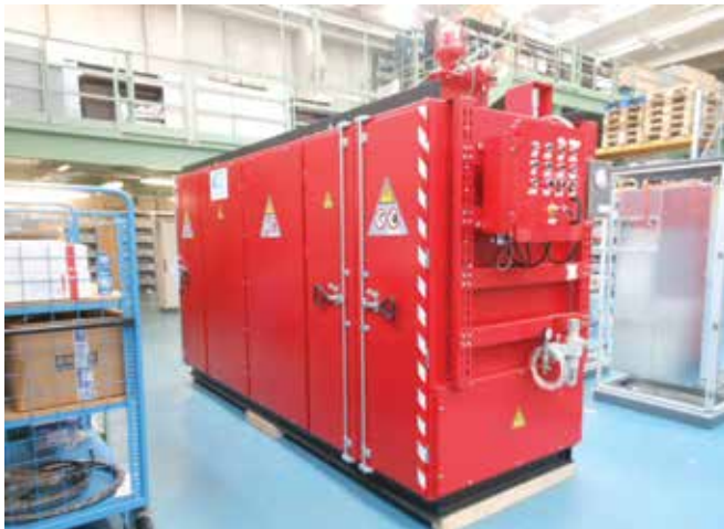
Fig. 3 - The prototype of Ex p substation
