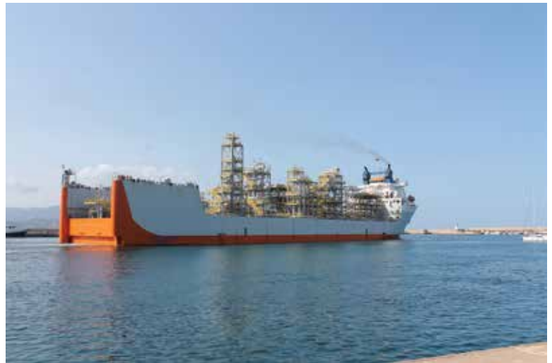
Fig. 7 - Sea transport of modules
