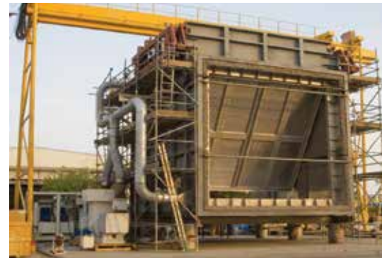
Fig. 2 - Amal 1C (Oman): diverter and guillotine dampers fully preassembled and tested in Oman
