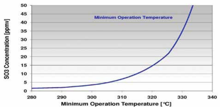
Fig. 4 – Diagram of catalyst Minimum Continuous Operating Temperature
