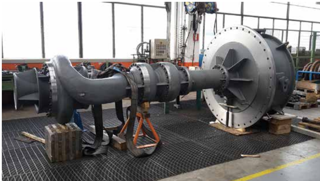
Fig. 2 – Booster pump assembly at Termomeccanica Pompe La Spezia workshop
