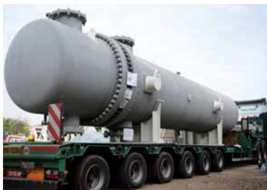
Fig. 2 - Shell & Tube heat exchanger (80 tons)
