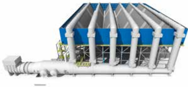
Fig. 3 – a) General arrangement ACC (Air Cooled Condenser) view; b) CT (Cooling Tower) design
