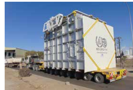
Fig. 3 - Rabab Arweel (Oman): diverter and guillotine dampers fully preassembled and tested in Oman
