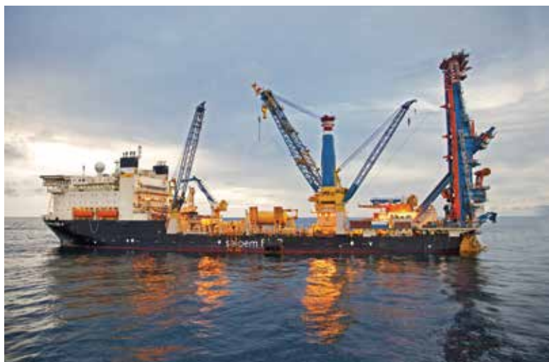
Fig. 2 - Saipem's J-lay and offshore construction vessel FDS2
