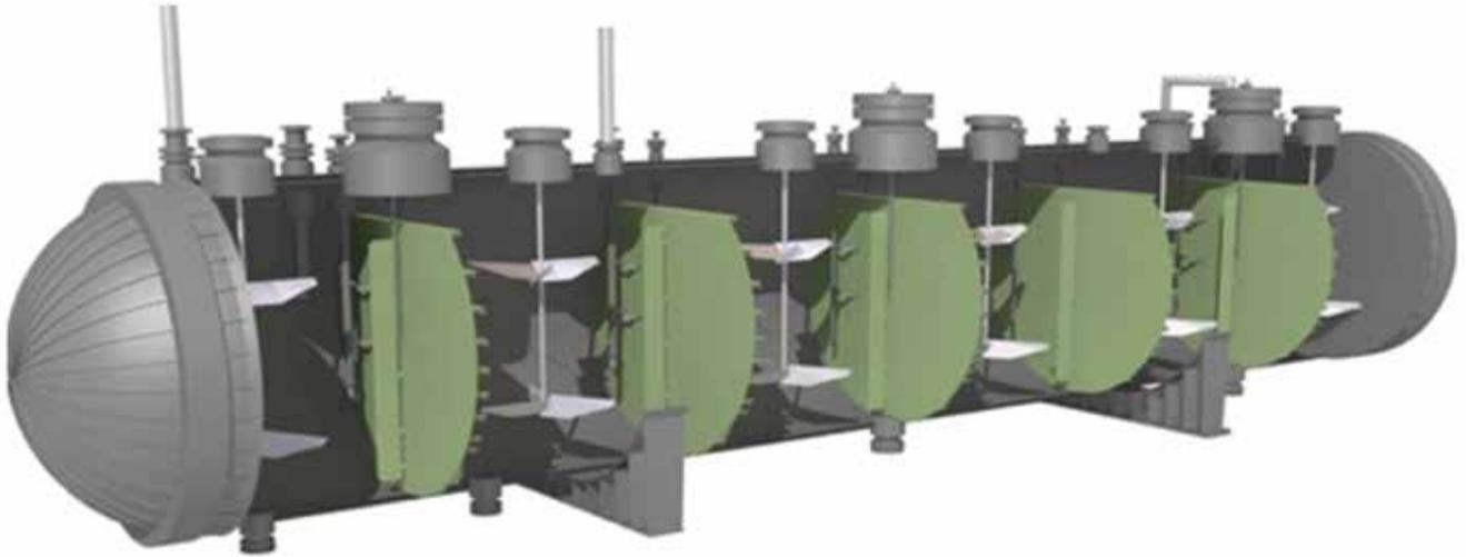
Fig. 6 – Autoclave for the rapid oxidation of the sulfide minerals
