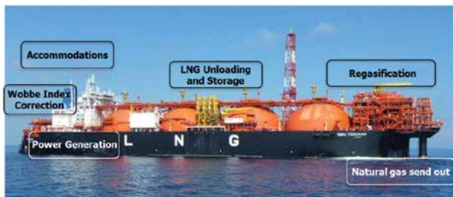
Fig. 1 - FSRU Toscana installed off-shore Livorno, Italy (courtesy of OLT)
