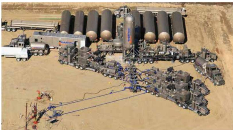
Fig. 4 - General view of GasFrac fracturing operation using liquid propane gas (from Montebourg 2015)
