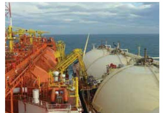
Fig. 6 - Loading arms connection to LNG Carrier (courtesy of OLT)
