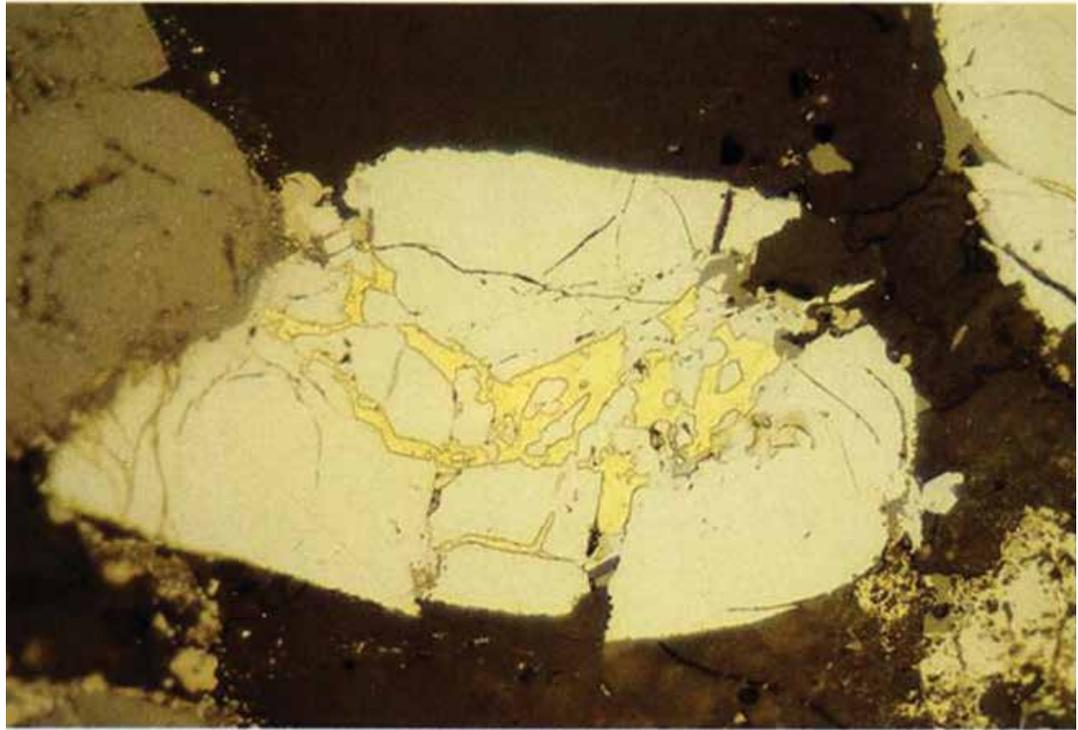
Fig. 3 – Gold in cracks in compact pyrite. Detrital uraninite (mid-grey), rimmed by brannerite, also occurs in the section. Basal Reef, Welkom mine (photomicrograph, linear magnification x 136)
