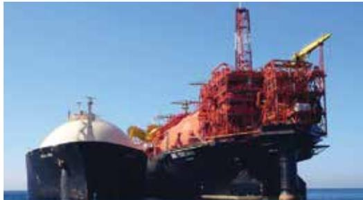
Fig. 5 - FSRU and LNG Carrier in side by side (courtesy of OLT).
