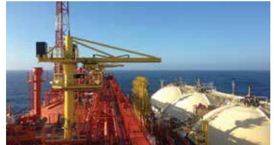
Fig. 6 - Loading arms connection to LNG Carrier (courtesy of OLT)
