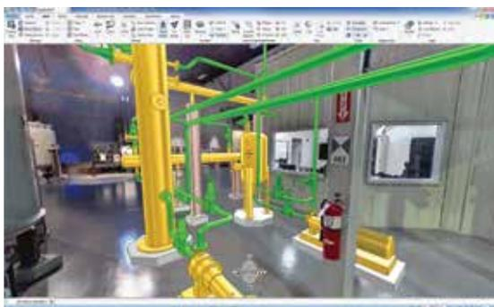
AVEVA E3D fuses the BubbleView photo-realistic laser scan data into the design environment enabling an as-is conditions of an asset
