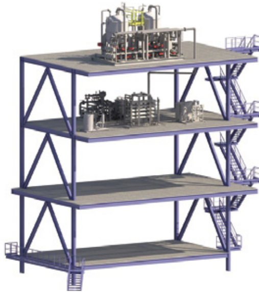
Figure 5. 3D Model of Membrane deaeration system
