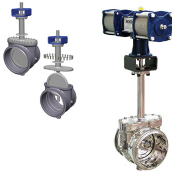
Figure 2: Cryogenic top entry TOVs offer an easily accessible trim that can be removed with the extended bonnet, making it safer to repair.
