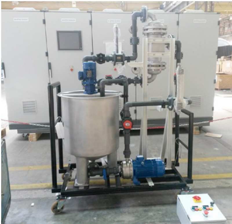
Figure 8. Pilot scale plant of solid - liquid hydrocyclone used for experimental campaign
