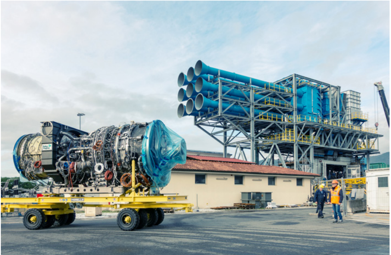
Baker Hughes' LM9000 gas turbine test bench
