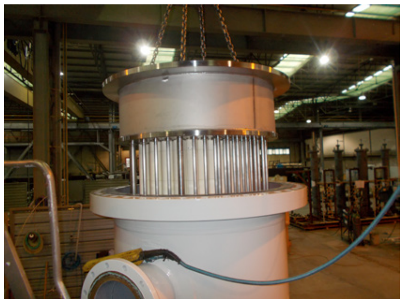
Figure 4 - Desanding cyclone manufactured in Cannon Artes factory before shipment to Congo
