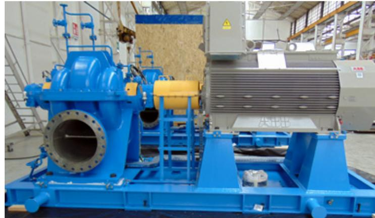
Pumps for Dubai's SWRO plant - TMP CPP pump model for sea water supply service (left) and DD pump model for water distribution service (right)
