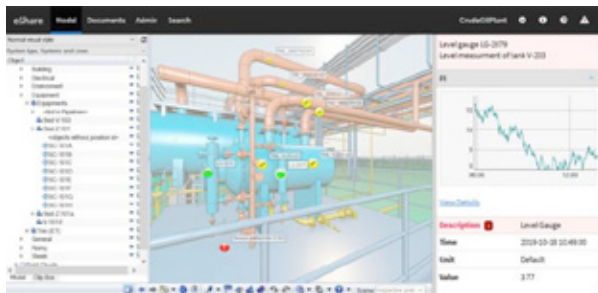
3D dashboard to constructability information – select model hierarchy according to building priority categories and color based on constructability analysis data
