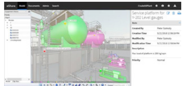
Collect notes from installation teams and use color-coding to visualize the installation status of the model in eShare
