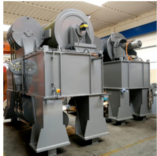
Picture of winches under constructions
