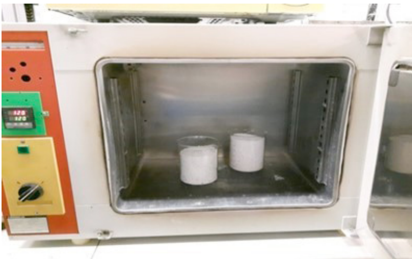
Figure 2. Activated alumina drying in oven @ 120°C.
