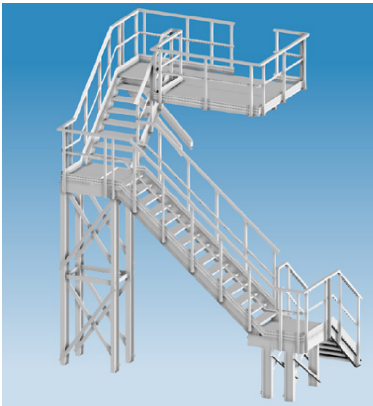
M.M. project regarding a FRP inclined stairway for tank access purposes
