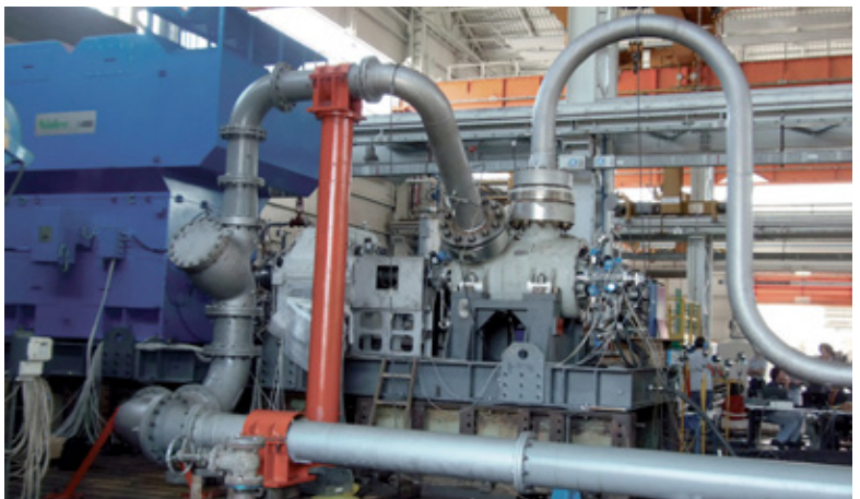
Termomeccanica Pompe API 610 BB5-type pump for water injection service at onshore oil extraction plant under final performance test at La Spezia in-house test center
