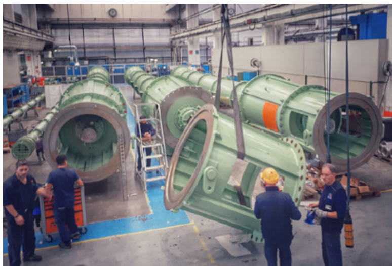
Termomeccanica Pompe API 610 VS1-type pump for sea water supply service at LNG regasification terminal
